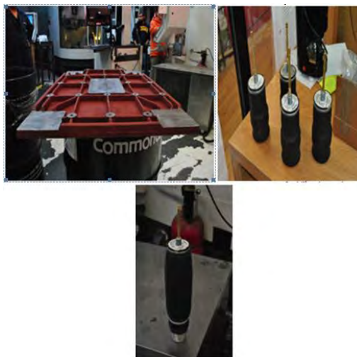
Figure 4 Finished ribbed plate and pneumatic legs for the vibratory table assembly
