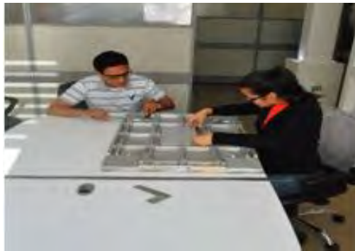
Figure 3 Patternmaking for foundry casting of the steeled vibratory table
